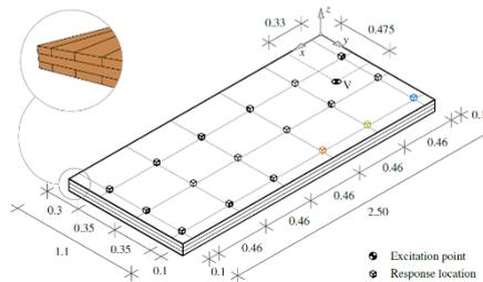
Figure 1: CLT plate with measurement setup.
