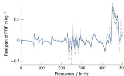
Figure 2: Measured FRF for the depicted CLT plate.
