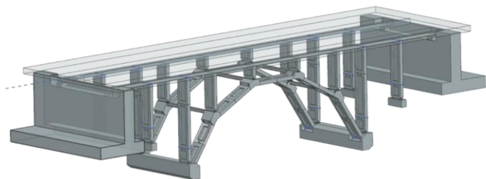
Figure 1: Sample Resulting Modular Bridge Model
