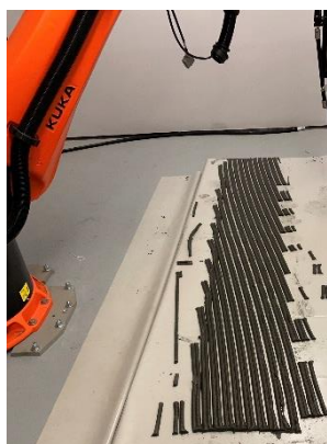
Figure 2: Manufacturing of concrete beams with an industrial robot by KUKA
