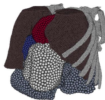
Figure 1.: Simulation of Total Artificial Heart to evaluate device fit
