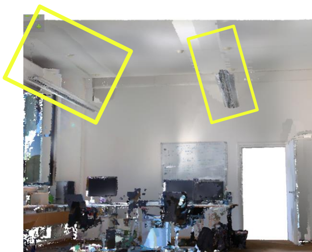
Point cloud missing points between ceiling and lamps (proximity criterion not satisfied)
