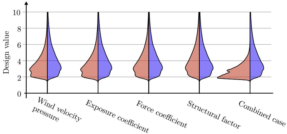
Figure 7: Violin plots showing the distribution of design values obtained with Eurocode models (blue) and advanced models (red).
