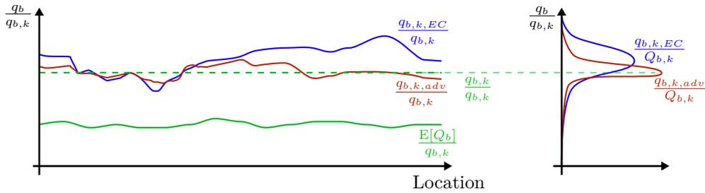
Figure 6: Re-illustration of Figure 5, whereby the wind velocity pressure  $Q_b$  (green) and the characteristic value according to Eurocode  $q_{b,k,EC}$  (blue) are standardized by the characteristic value of the aleatoric distribution. The characteristic value according to advanced modeling techniques  $q_{b,k,adv}$  is added in red.
