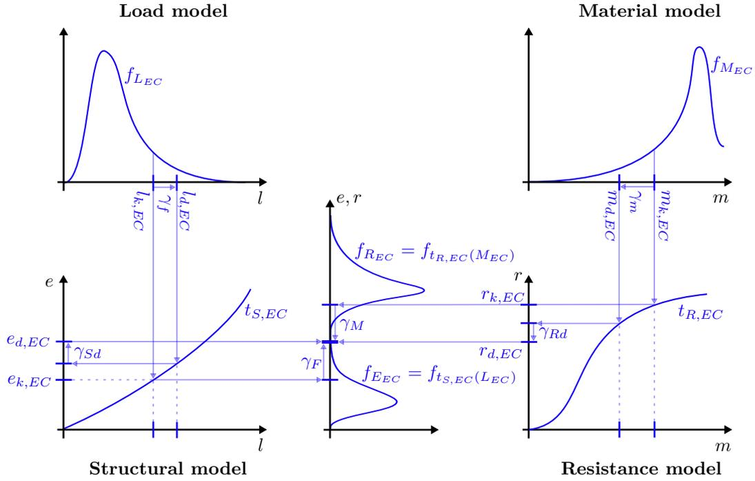
Figure 3: Illustration of the basic reliability problem and its relation to Eurocode models.
