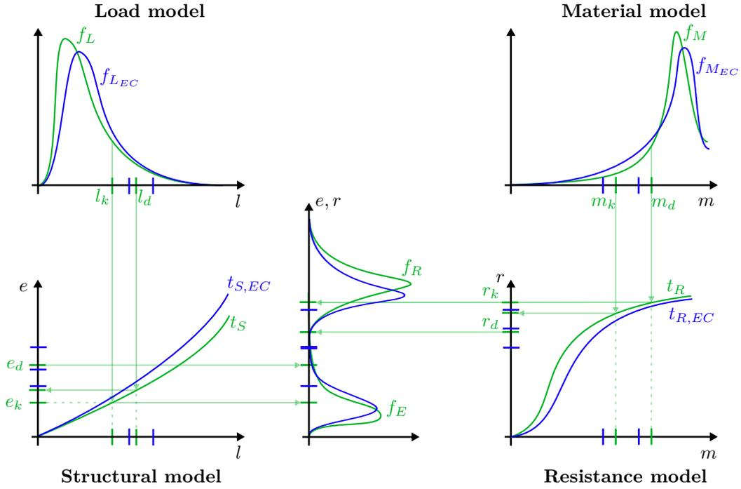
Figure 4: Illustration of the Design approach of the Eurocode (blue) compared to the purely aleatoric models (green) for one specific design situation.
