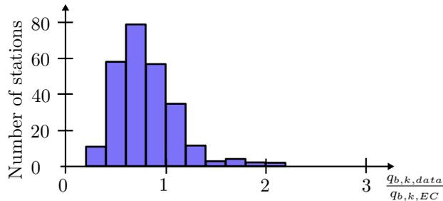
Figure 9: Histogram of the ratios of the characteristic values  $q_{b,k,Data}$  obtained from data of the German Meteorological Service [57] and the characteristic values  $q_{b,k,EC}$  of the respective location specified in the Eurocode [45].
