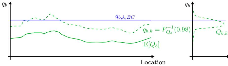
Figure 5: Exemplary illustration of the derivation of the distribution of the characteristic value  $Q_{b,k}$  resulting from the aleatoric distribution of the wind velocity pressure  $Q_b$  (green) and its relationship to the characteristic value according to Eurocode  $q_{b,k,EC}$  (blue).
