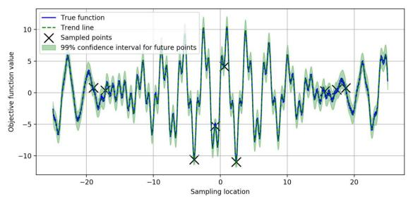
Predictive distribution for future sampling points of a complex objective function that presents difficulties when optimized with commonly utilized methods after 9 previously sampled points. In this case, frequencies of the harmonic functions making up the objective function were assumed to be known in advance.
