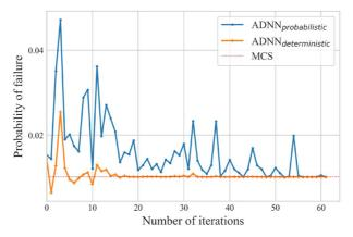
The graph displays estimated probability of failure by the proposed ADNN-MCS method, plotted over the number of active learning iteration steps. The orange and blue curves show predictions when DNN's prediction is considered deterministic or probabilistic, respectively. Active learning is stopped if the DNNs' prediction reaches a predefined threshold of confidence; this often coincides with when the two predictions show a marginal difference.
