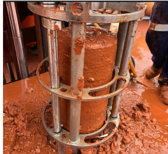
Figure: Use of the type Mini-block Sampler (Black Insitu Testing, Australia) as an example of advanced sampling techniques
