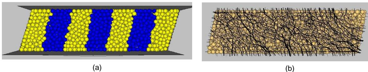
**Figure 1: (a) Simulated simple shear specimen of glass beads at 20% shear strain (b) Simulated force chains of glass beads at a shear strain of 20% (Dabeet 2014)**
