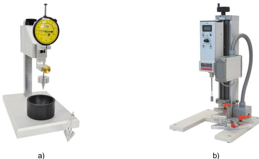
Figure: Laboratory tests equipment for cohesive soils a) Fall Cone test b) Vane Shear test
