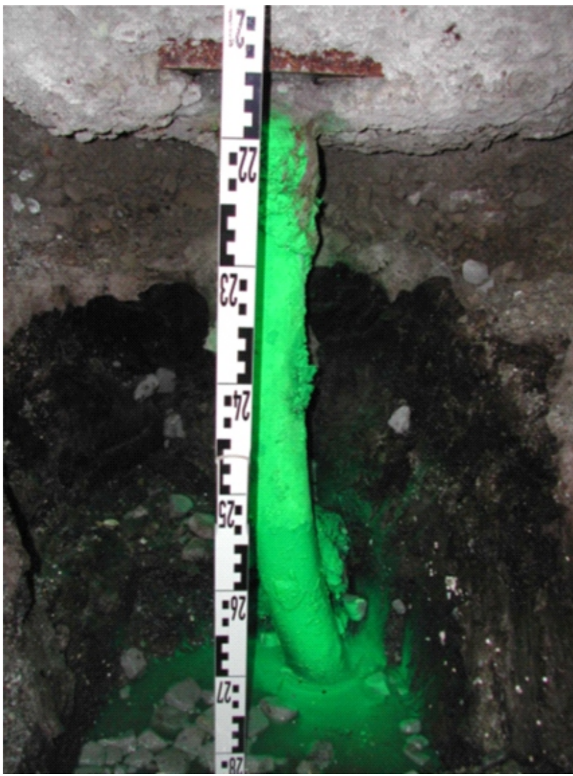
Stabilitätsversagen eines Pfahles und Dokumentation eines Schadensfalles Damaged pile by the loss of stability and the resulting large settlement
