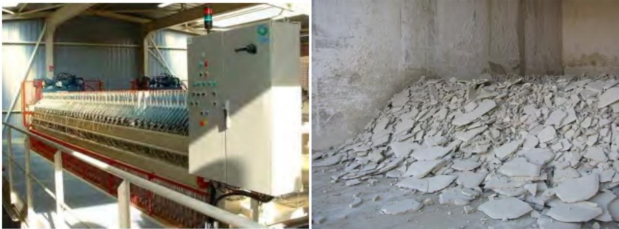
Figure 8: Filter press and chalk “plates” after dewatering
