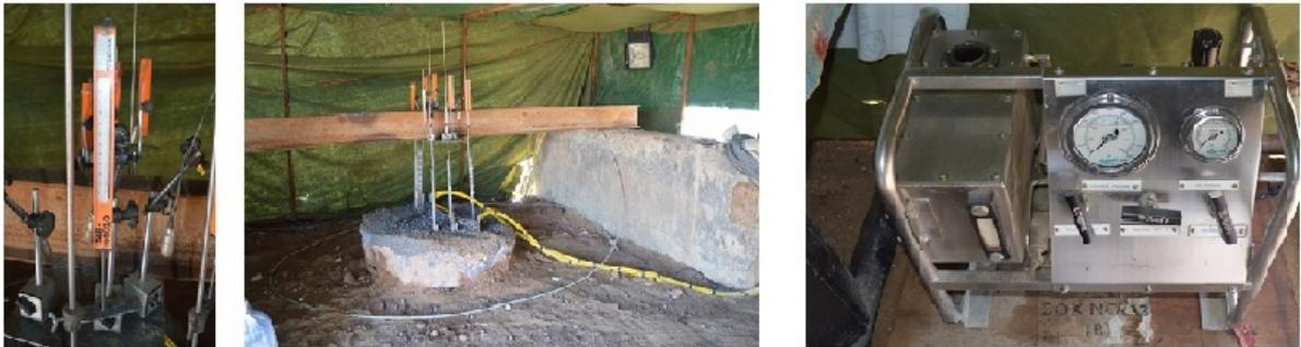
Figure 8: O-cell tests of piles in construction site Expo (Astana, Kazakhstan)
