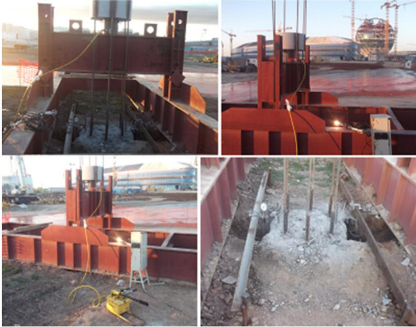
Figure 5: Vertical pulling load test (Astana)
