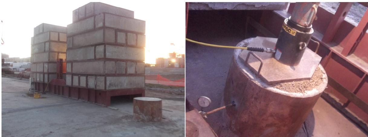
Figure 3: Photo of static load testing in Kazakhstan (Astana)
