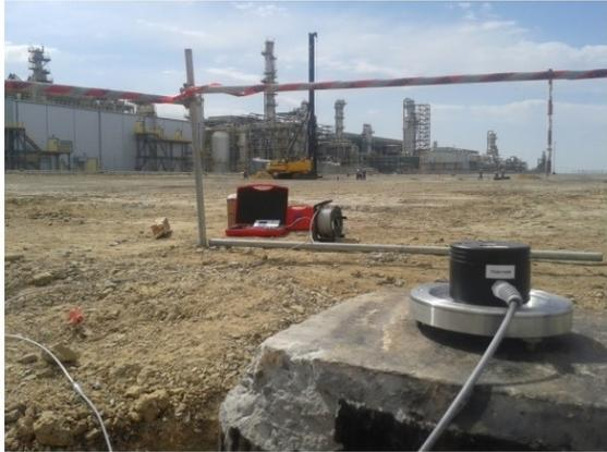
Figure 12: Vibration monitoring at the Tengiz oil and gas facilities (West Kazakhstan)
