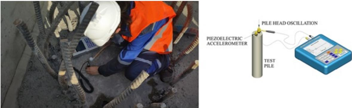
Figure 10: Photo and schema of pile integrity testing in Kazakhstan (Abu-Dhabi Plaza, Kazakhstan)
