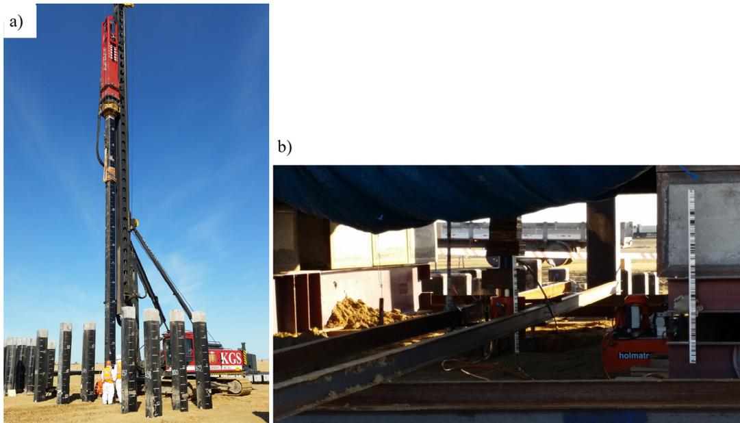
Figure 2: Photo pile testing: a) Dynamic load testing (DLT- driving pile) b) Static load testing (SLT-driving pile)
