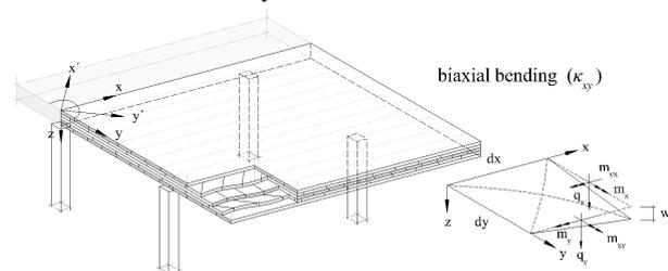
Fig. 2: Biaxial load transfer of DLT elements with point-supports
