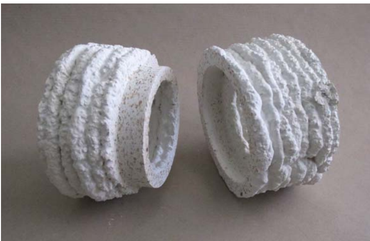
Figure 5: Subtractive finishing of additive manufactured test objects from wood concrete (sample fabricated by S. Stanglmayr)
