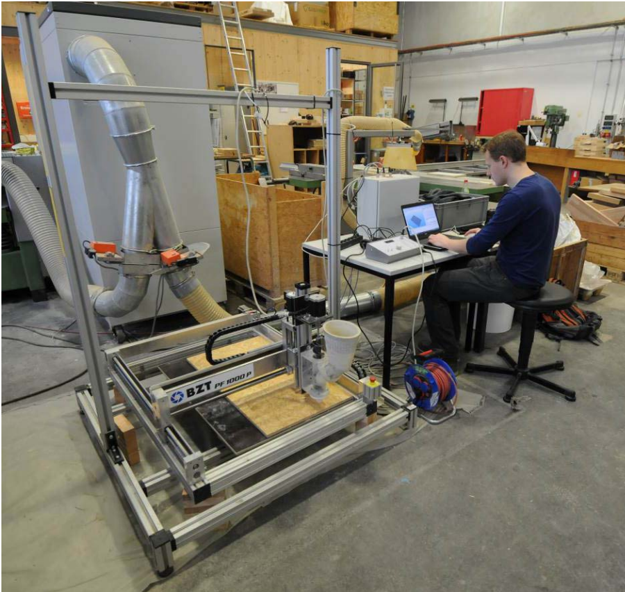
Figure 3: Gantry system with mounted extruder
