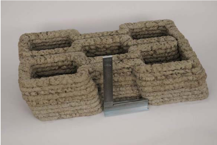
Figure 4: Extruded wood concrete test object with overhang
