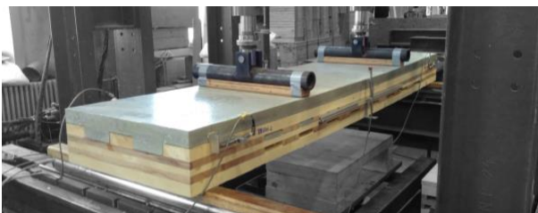
Figure 8: TCC specimen under bending in the test facility
