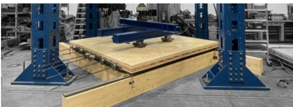
Figure 7: Prestressed specimen under biaxial bending in the test facility
