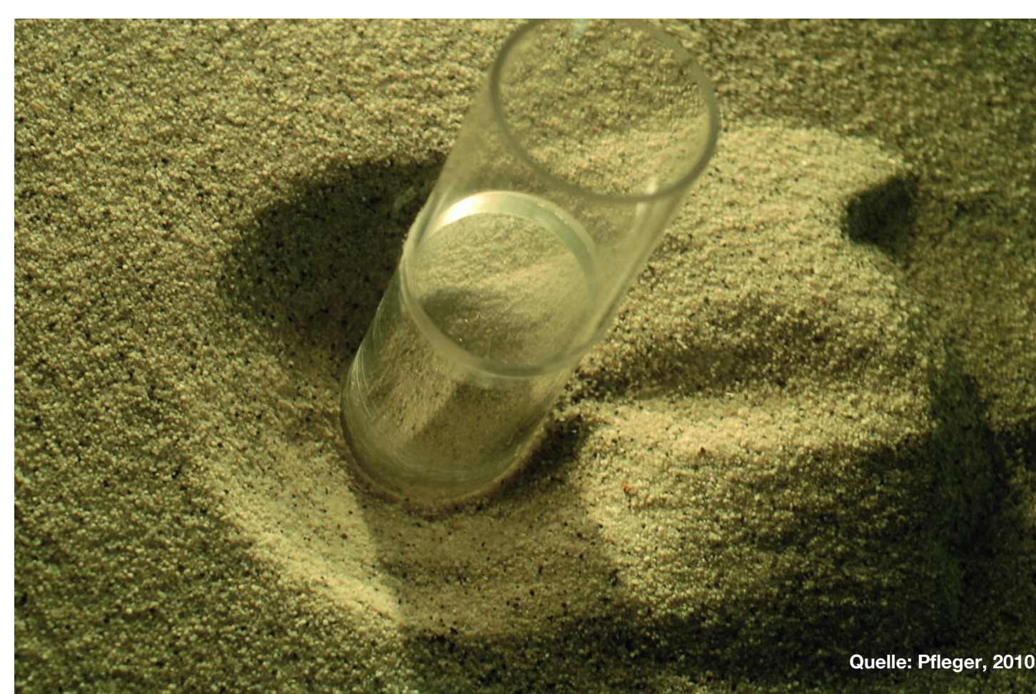
Scour hole around a cylinder in a sandy bed. Photograph taken during the experiments in the Chair's Laboratory, (Pfleger et al., Int. Conf. Scour & Erosion, 2011).
