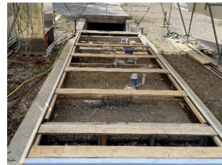
Abb. Existing 2D-model aquifer for experiments in Obernach
