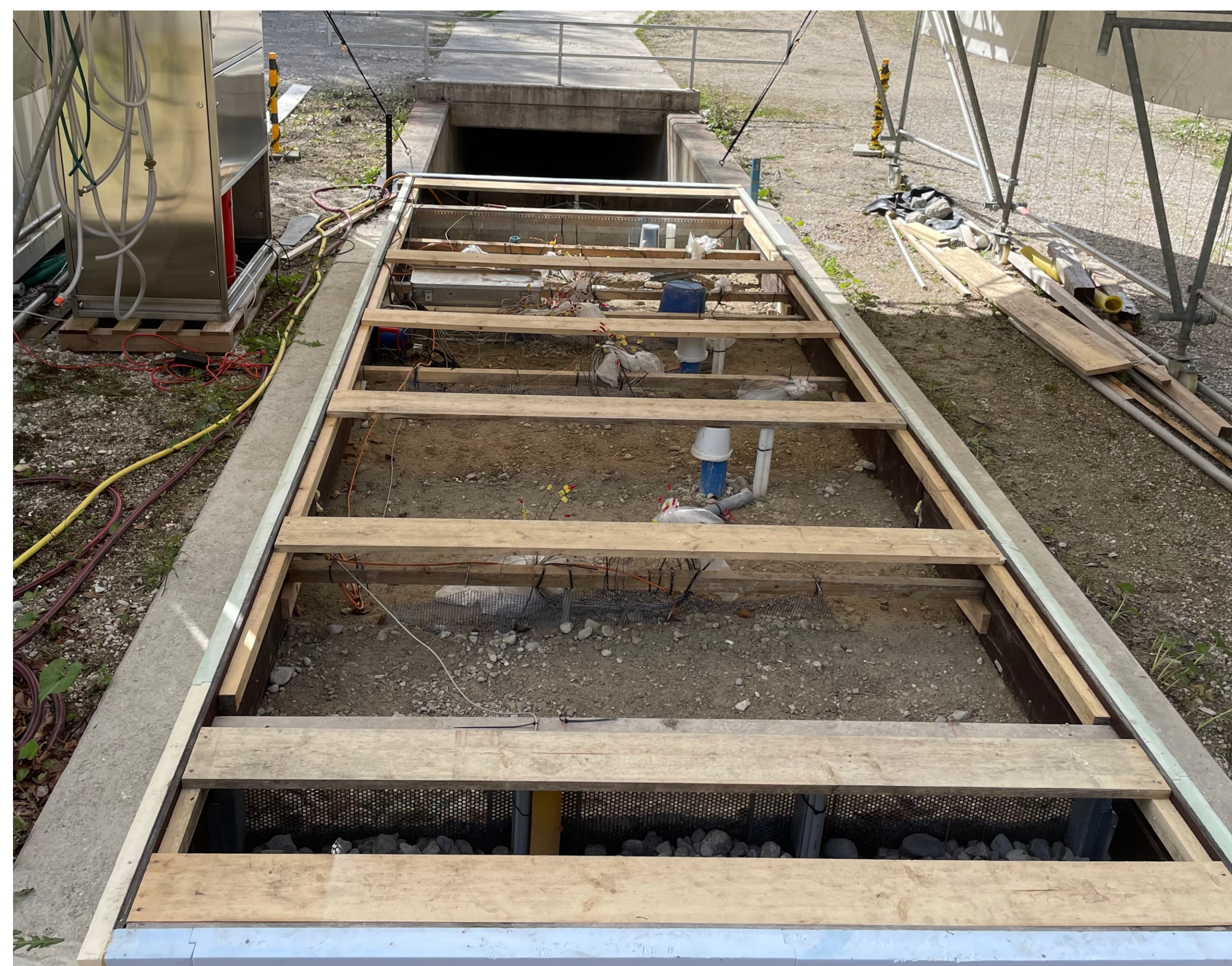
Fig. 1: Illustration of the flow-through tank in the Oberrach test centre of the TU Munich.
