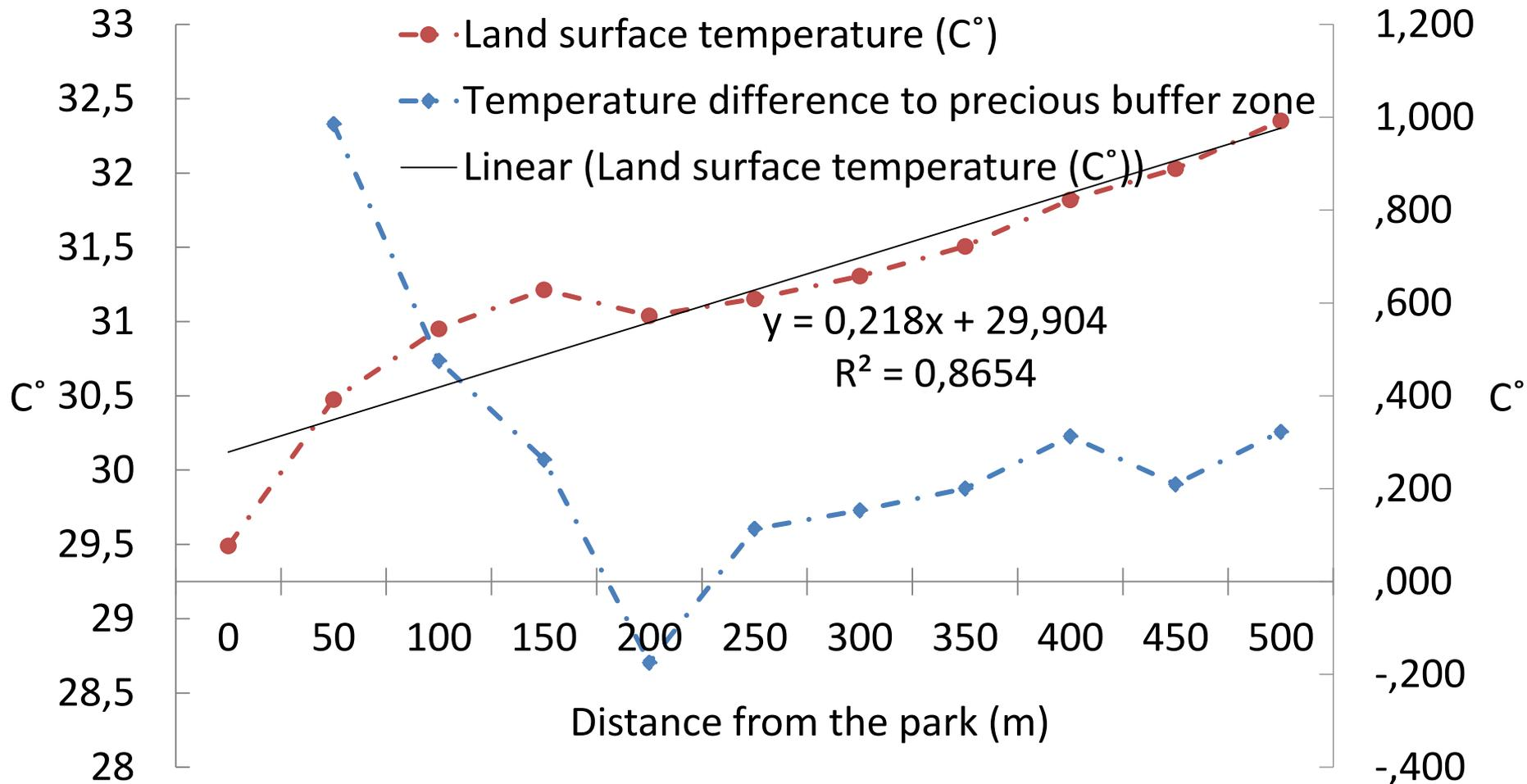
Average land surface temperature variations of buffer zones (primary vertical axis) and temperature difference to previous buffer zone (secondary vertical axis)
