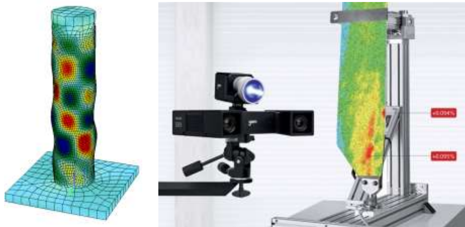
Figure 1: Left: first buckling mode based on a linear prebuckling analysis of a stub-column-test in SOFiSTiK;right: example of a optical shape change analysis 1
