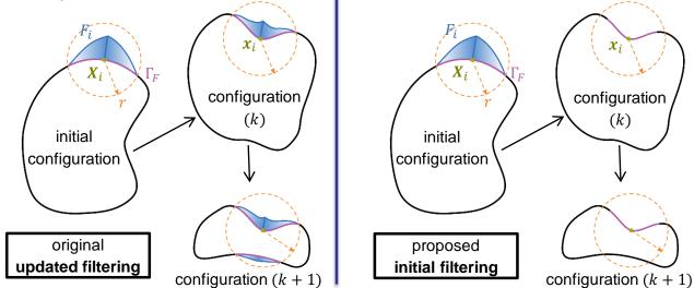
The original formulation by [Hojjat] updates the filtering operation according to the new geometry configuration, and hence constructs a non-linear relation between the design control variables and the physical shape. Strictly mathematically speaking this leads to an alteration of the initial optimization problem after each shape change.
