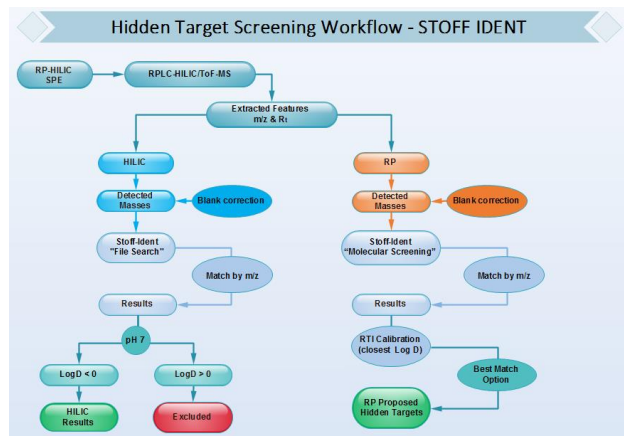
Fig. 1: Hidden Target Screening workflow using STOF-IDENT Database
