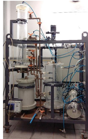
Fig. 2: Bench-scale AnMBR with two reactors in series for vinasse treatment.
