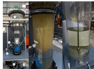
Fig. 1: Ultrafiltration test-skid for municipal wastewater treatment.
