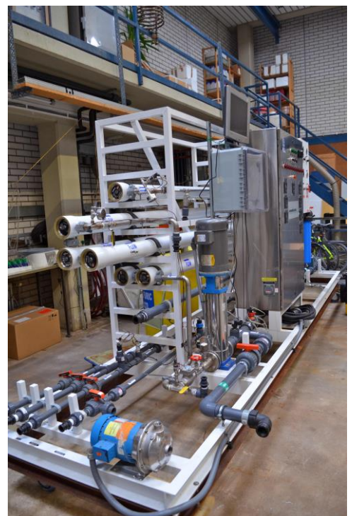
Figure 1: Pilot-scale nanofiltration test skid (80 L/min)
