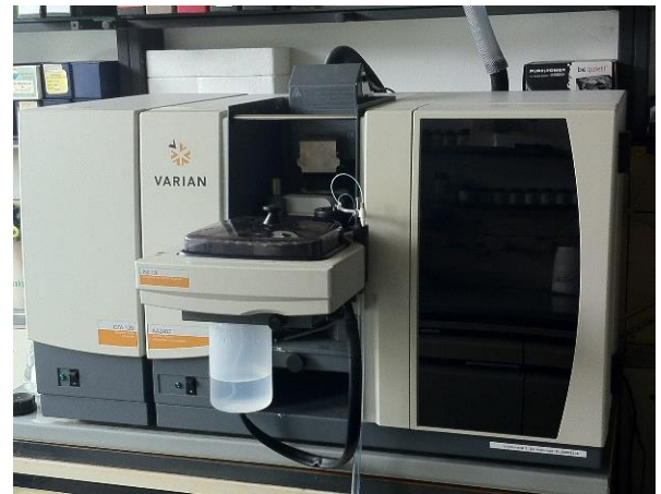
Figure 2: Graphite furnace AAS for the analysis of metals
