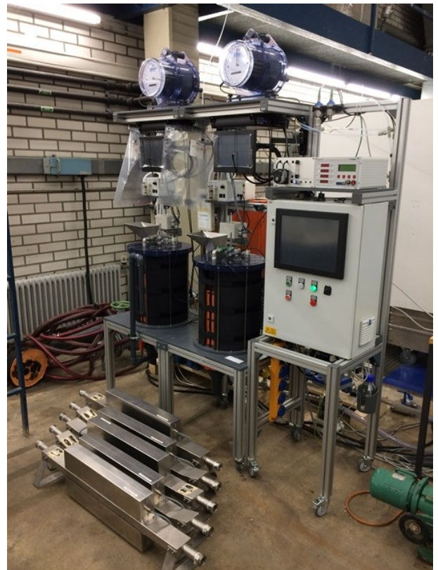
Figure 11: Continuously operated digesters with ultrasound test systems
