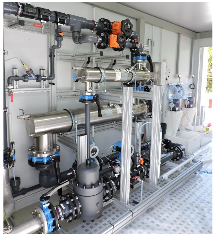
Figure 32: UV/H 2 O 2 pilot plant at WWTP Gut Marienhof (Munich II)
