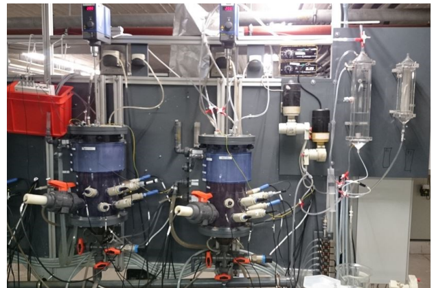
Figure 8: Automated bio reactor system according to the design at EAWAG
