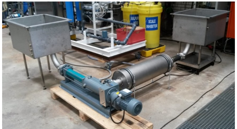
Figure 6: System for the treatment of sewage sludge by ultrasound
