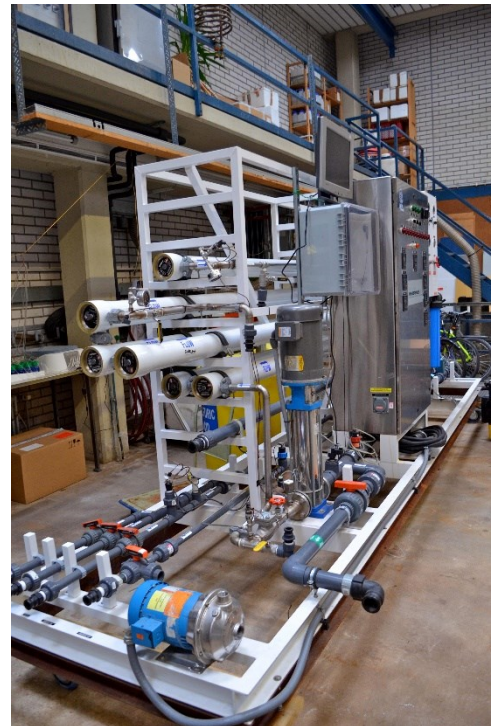
Figure 1: Pilot-scale nanofiltration test skid (80 L/min)
