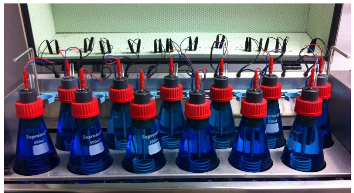
Figure 2: Sapromat for the analysis of the biological oxygen demand (BOD)
