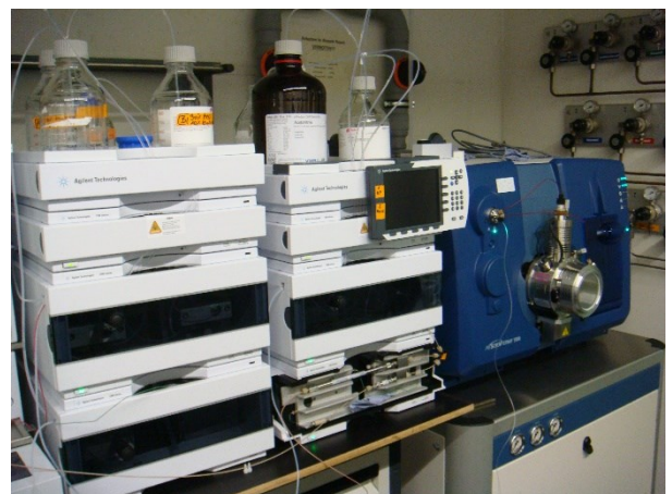
Figure 3: LC/MS-MS System for analysis of trace organic chemicals at the sub ng/L level
