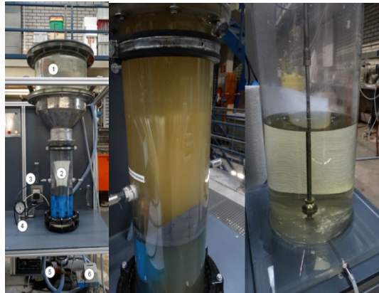
Figure 27: Ultrafiltration test-skid for municipal wastewater treatment
