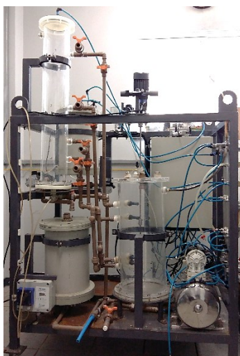
Figure 30: Pilot-scale anaerobic MBR with two reactors in series for vinasse treatment.
