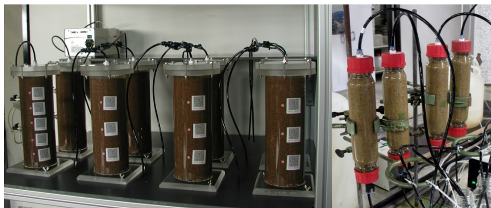
Figure 22: Different setups for soil column experiments
