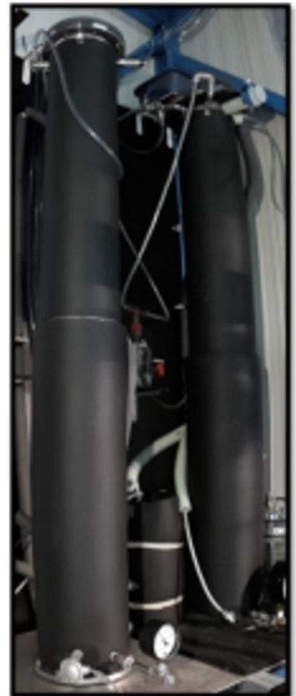
Figure 10: Trickle bed reactors at pilot plant scale
