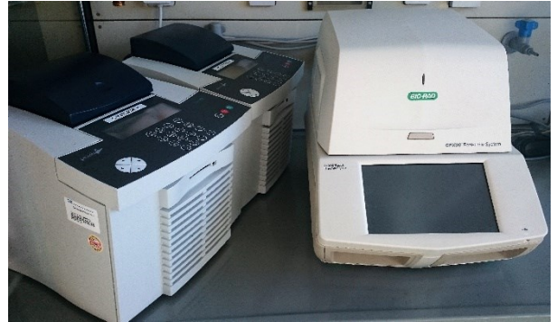
Figure 4: PCR and qPCR systems to amplify and quantify different genes of interest
