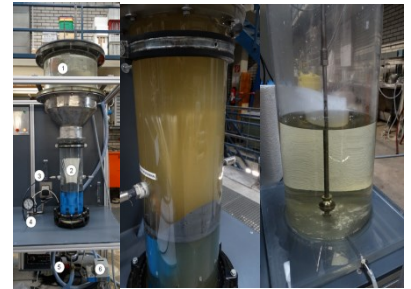
Fig. 32: Ultrafiltration test-skid for municipal wastewater treatment.
