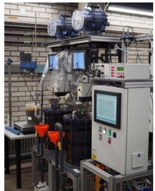
Fig. 7: Continuously operated biogas reactor.
