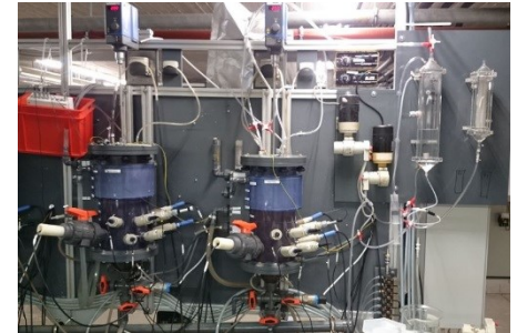
Fig. 8: Automated bioreactor system according to the design at EAWAG.
