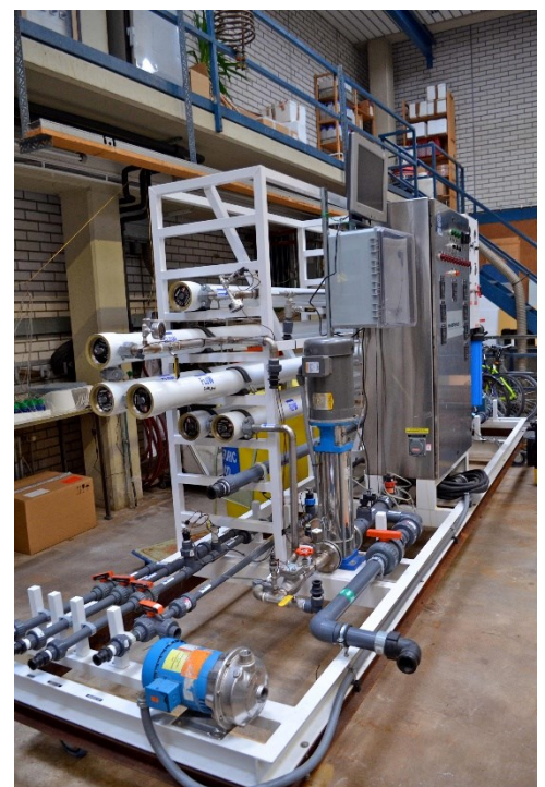
Fig. 1: Pilot-scale nanofiltration test skid (80 L/min).
