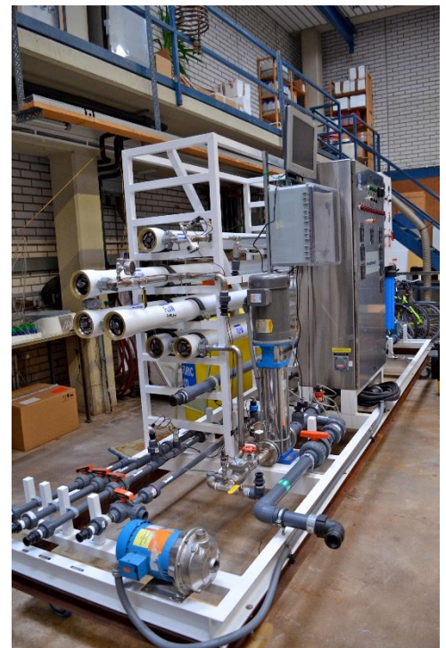
Fig. 1: Pilot-scale nanofiltration at 80 L/min
