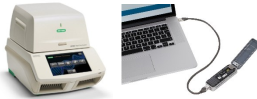
Fig.31: qPCR Analysis targeting different antibiotic resistance genes and a third generation sequencing based handhold sequencer for analyzing marker genes, microbial genomes and metagenomes
