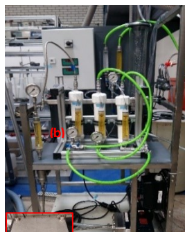
Fig. 28 Bench-scale RO membrane system with a flexible configuration: (a) flat sheet or (b) spiral-wound module.
