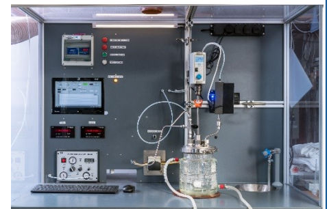
Fig. 14: Bench-scale ozonation system
