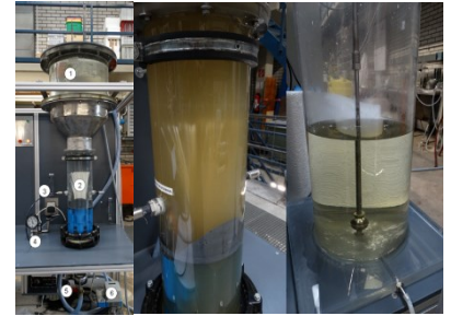
Fig. 25: Ultrafiltration membrane for municipal wastewater treatment.
