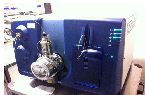
Fig. 3: LC-QTRAP-MS system by AB Sciex for trace analysis
