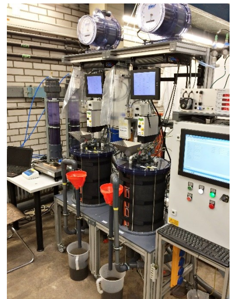
Fig. 11: Continuously operated biogas test system
