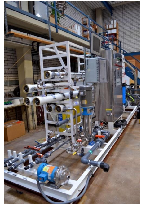
Figure 1. Pilot-scale nanofiltration test skid (80 L/min).
