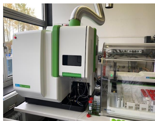
Figure 2. Determination of heavy metals using ICP-OES by Perkin Elmer.
