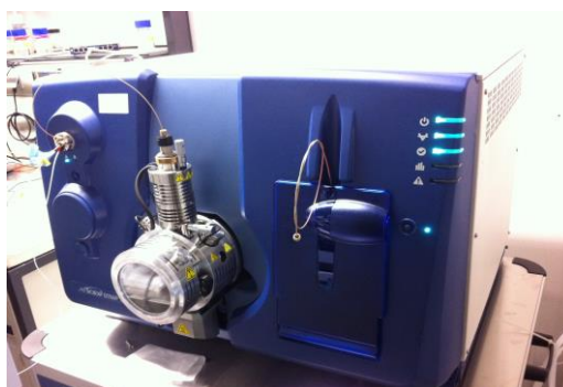
Figure 3. LC-QTRAP-MS system by AB Sciex for trace analysis
