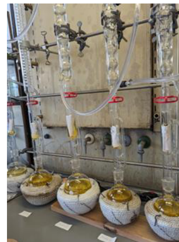
Figure 45. Soxhlet extraction of the solid phase of ADS.
