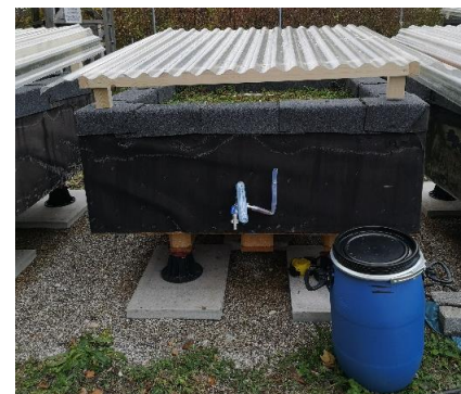
Figure 8. Experimental setup of semi-technical scale leaching experiments. Left: Different combinations of root barriers (physical, chemical) and roof types (gravel, extensive- and intensive green roof), Right: Intensive semi-technical green roof for experiments
