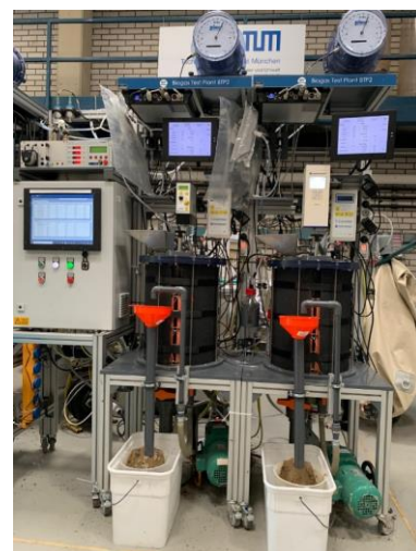
Figure 12. Continuously operated reactors on a pilot plant scale.
