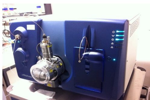
Figure 3: LC-QTRAP-MS system by AB Sciex for trace analysis.
