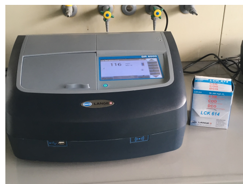
Figure 2: Determination of single and sum parameters through cuvette tests using the HACH-photometer.
