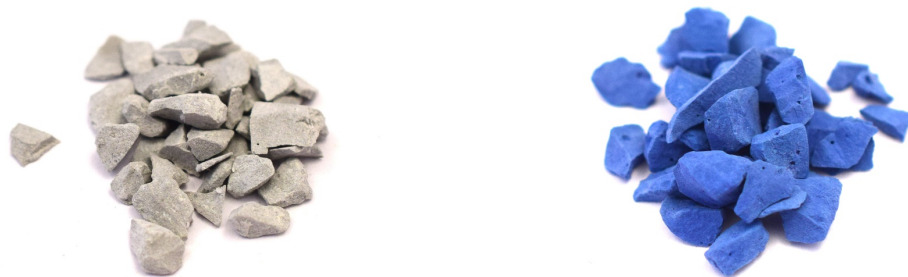
Figure 27: Hardened cement granulates before (left) and after (right) exposure to Reactive Blue 19.
