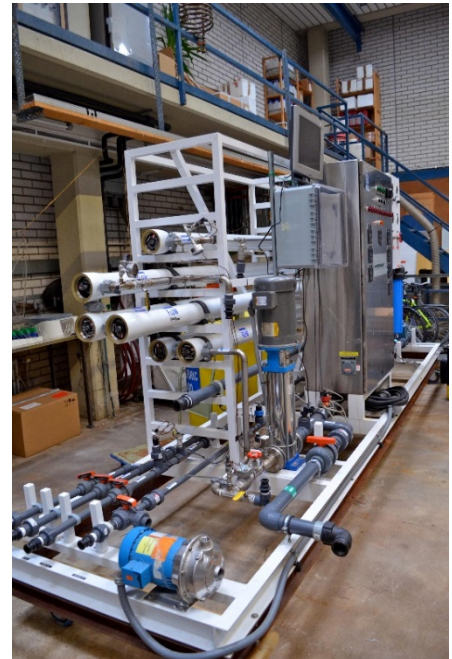
Figure 1: Pilot-scale nanofiltration test skid (80 L/min).
