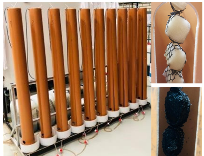
Figure 42: DHS reactor sketch and picture of whole experimental setup and clean as well as overgrown polyurethane sponge filling material.
