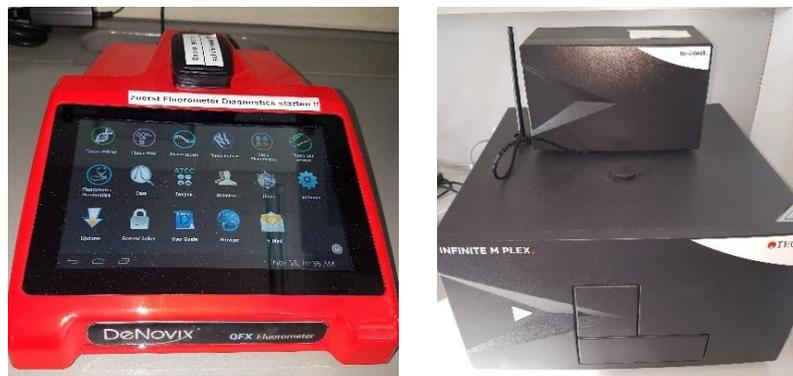
Abbildung 7: Links: DeNovix QFX Fluorometer; Rechts: Infinite M Plex Plate Reader von Tecan
