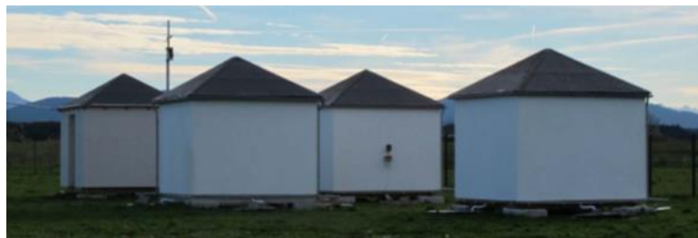
Figure 11: Specimens of outdoor leaching tests in Fraunhofer-IBP (Valley, Germany)
