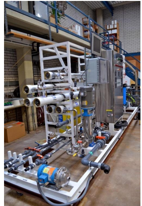
Figure 1: Pilot-scale nanofiltration test skid (80 L/min)
