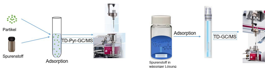
Figure 37: Particle analysis with TD-Pyr-GC/MS (left) and with Gerstel Twister® (right)
