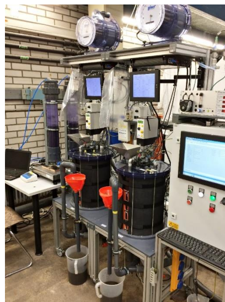
Figure 17: Continuously operated biogas test system
