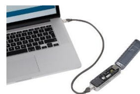
Figure 30: qPCR Analysis targeting antibiotic resistance genes, and a third generation sequencing based USB sequencer for analyzing marker genes, genomes and metagenomes
