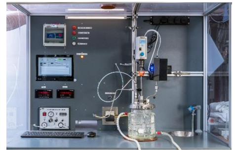
Figure 20: Bench-scale ozonation system
