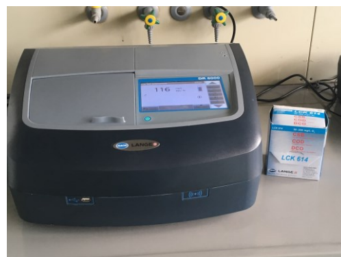
Figure 3: Determination of single and sum parameters through cuvette tests using the HACH-photometer.
