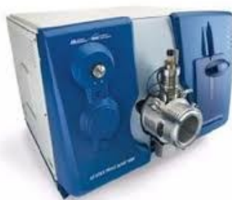
Figure 34: Left: AB Sciex QTRAP 5500 mass spectrometer for the identification of transformation products. Right: Example for the formation of transformation products during ozonation.
