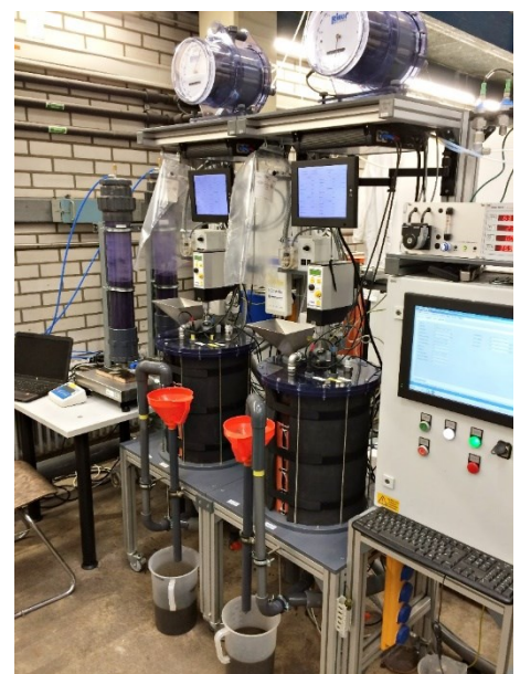
Figure 13: Continuously operated biogas test system.
