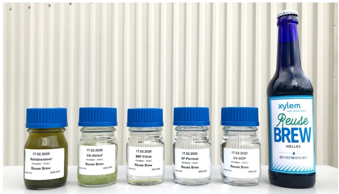
Figure 25: Water samples of the different treatment steps as well as the finished beer.
