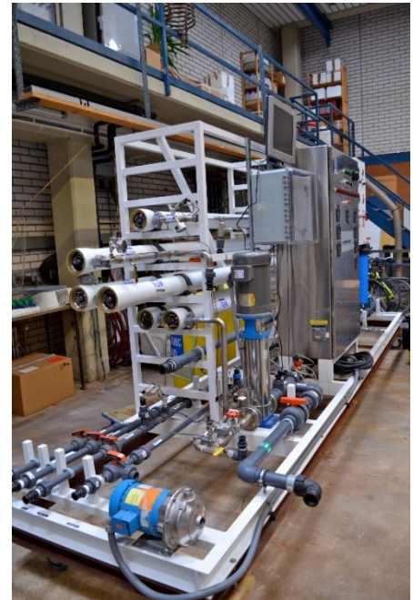
Figure 1: Pilot-scale nanofiltration test skid (80 L/min).
