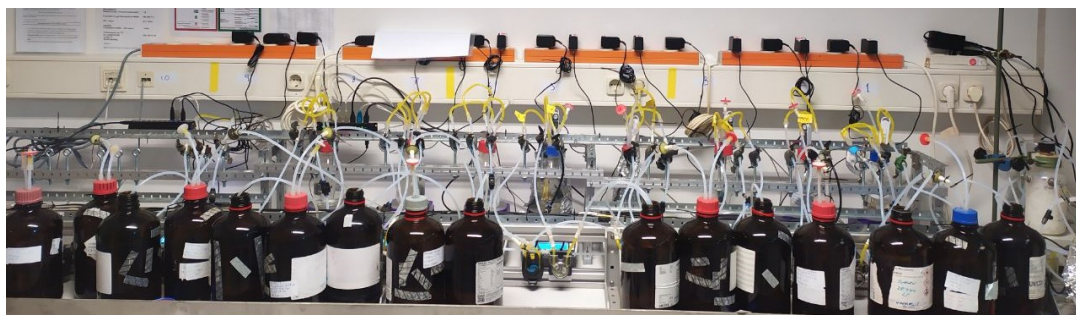
Figure 22: Current experimental set-up able to run 10 experiments in parallel.
