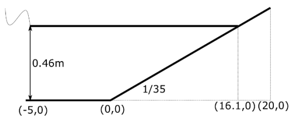
Figure 3 Bottom configuration for the test case of constant slope.
