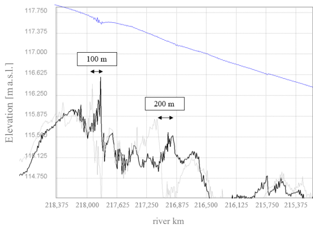
Figure 10. Moving bed formations before (grey) and after (after) 70 days of simulation.
