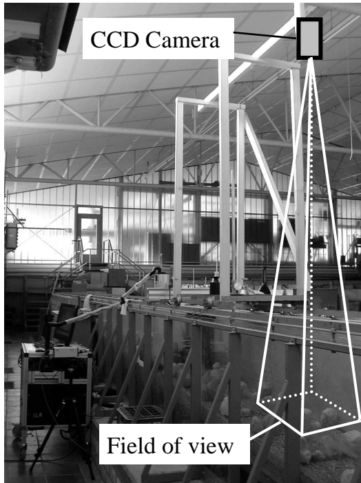
Fig. 3.4.16: Installation of PIV-facilities to measure the surface velocity distributions
