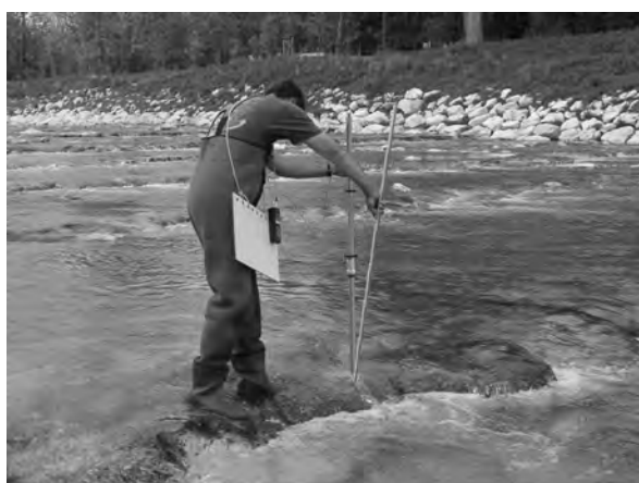
Fig. 4.4.15(a): Using midi-current-meter and ruler to measure the near bottom velocity and geometry of openings at boulder sills.
