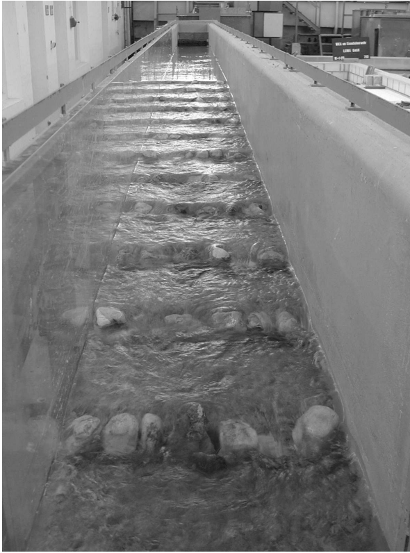
(a) The rough channel with boulder sills, view from downstream
