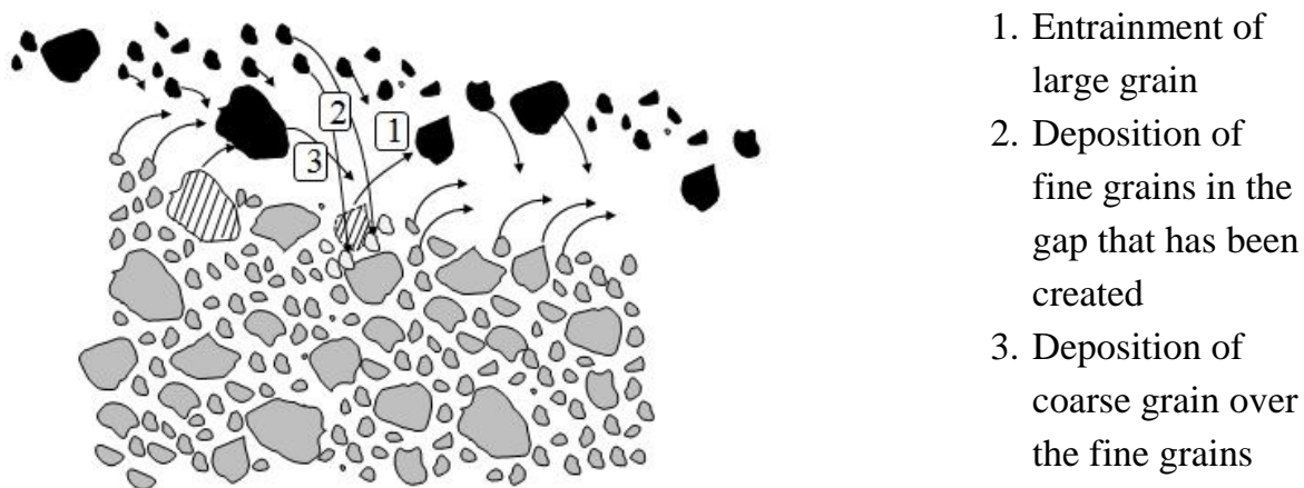
Fig. 2.4 Explanation sketch for mechanism of vertical winnowing
