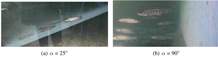
Figure 3.5 Brown trout at the 25^\circ inclined screen (a) and at the vertical screen (b)
