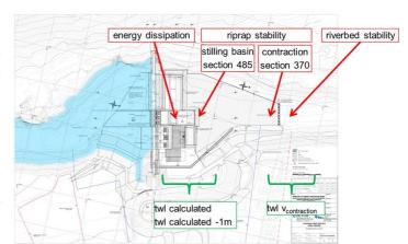
The spillway and the bottom outlet are followed downstream by a stilling basin followed by a riprap of 115 m length in a river contraction.
