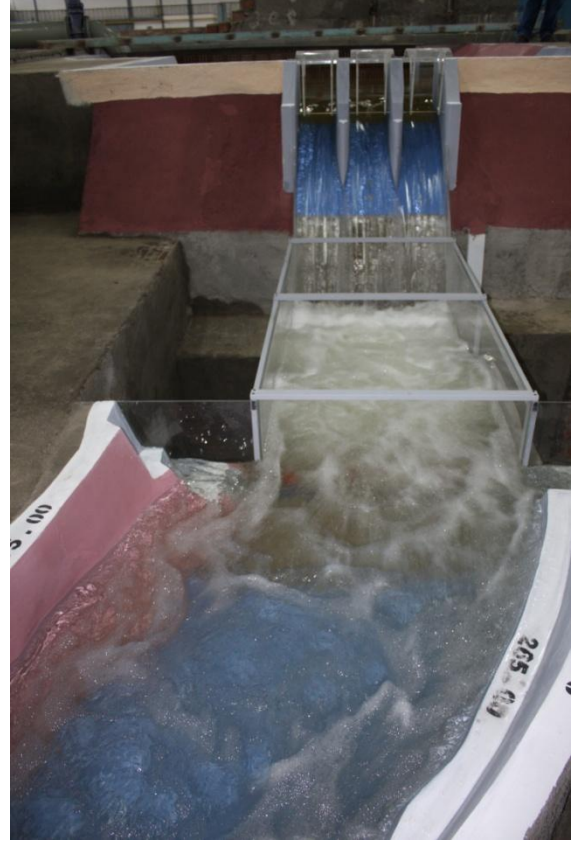
Figure 2: The physical model under operation ( Q=3856 \text{ m}^3/\text{s} -original design)
