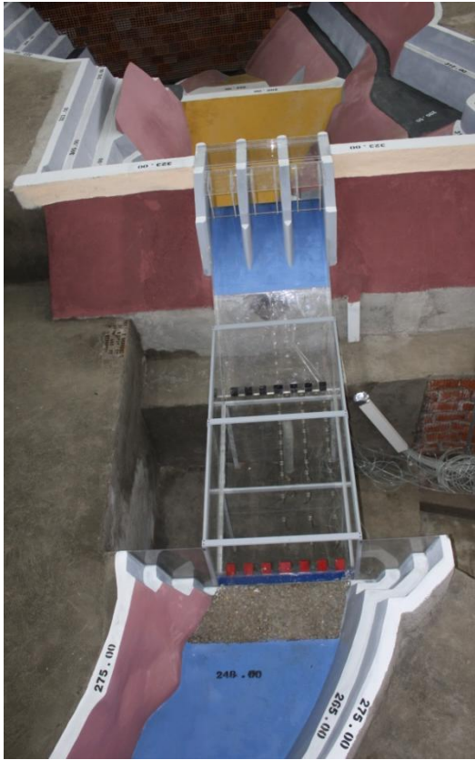
Figure 1: View of the 1/50-scaled physical model (original design)
