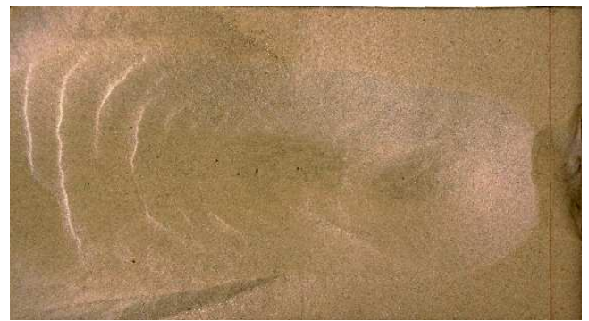
Figure 9: Scour geometry resulting from Kaplan propeller with double rudder.
