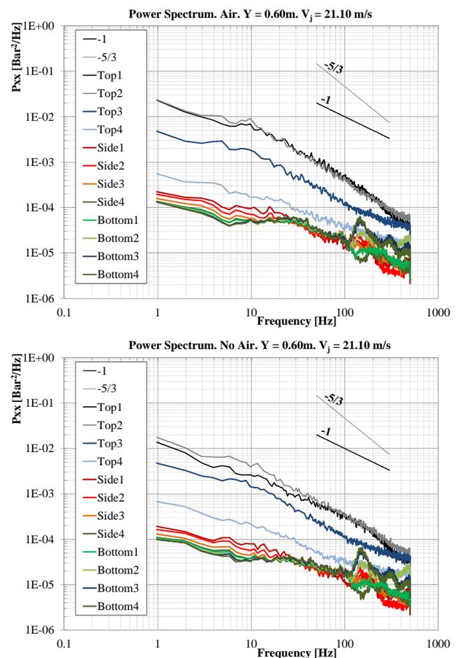
Figure 7: PSD plots for developed jets, with entrained air (top) and without entrained air (bottom).
