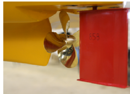
Figure 4: View of the Wageningen-propeller with central rudder.
