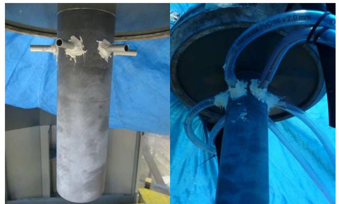
Figure 3: Photos of the nozzle with aluminium tubes installed for air entrainment. In the left, flexible tubes for measurement of entrained air
