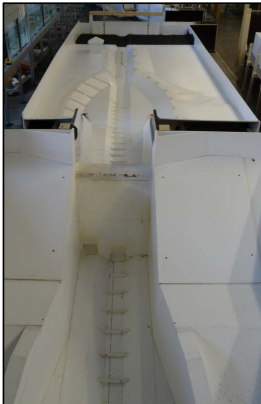
Figure 1: physical model, view downstream with corridor, outlets, spillway and depression shaped plunge pool
