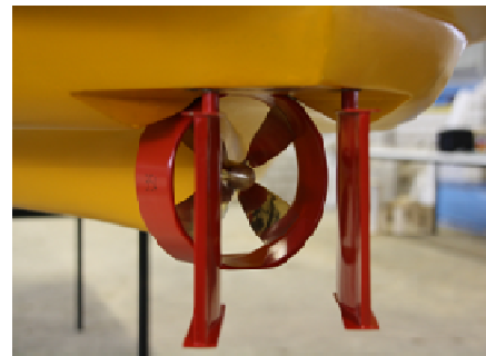
Figure 3: Kaplan propeller in a Kort nozzle with double-rudder.
