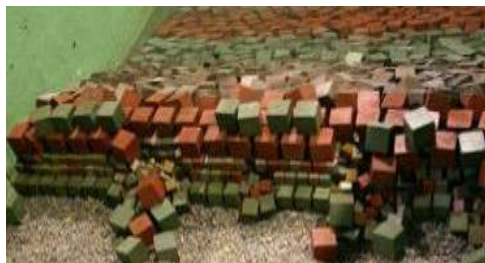
Figure 1. Stage 2. Crown failure ( H_s = 11 m; T_p = 20 s)
