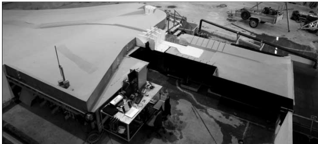
Figure 1 – Overview of the physical model of Hvammur HEP in the laboratory.
