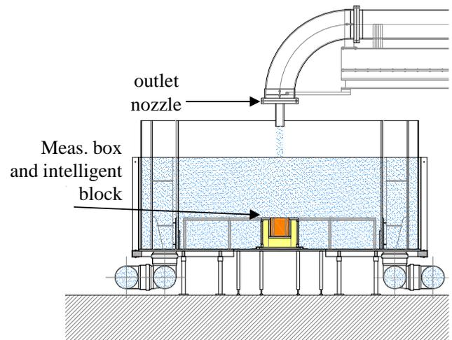
Figure 2: Side view of the experimental facility (Federspiel et al. 2009)
