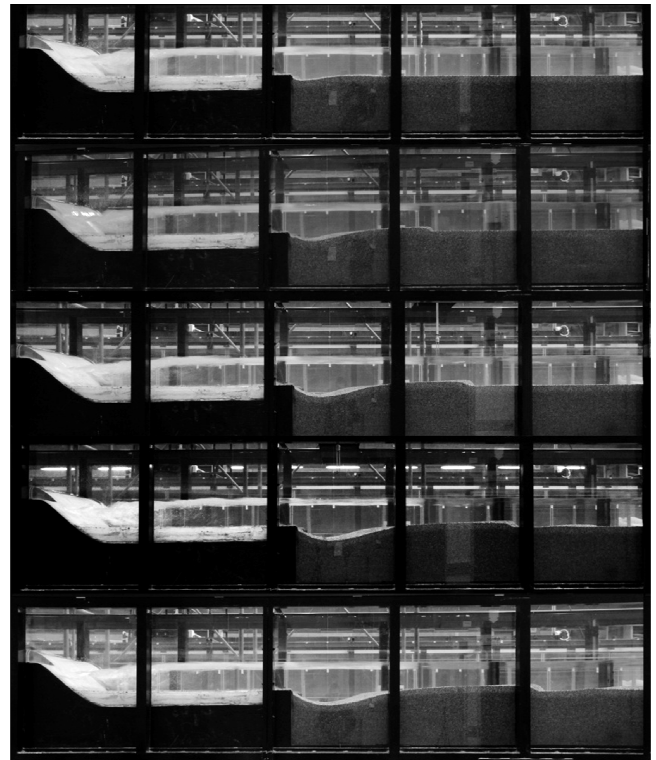
Figure 2: Hydraulic and bed morphology features with time for run C16 with discharge Q=60 l/s, tailwater depth h_{tw}=0.21 m and d_{50}=1.7 mm. Photographs from the top to the bottom refer to times t=2, 12, 24, 48 , and 72 hours from run starting.
