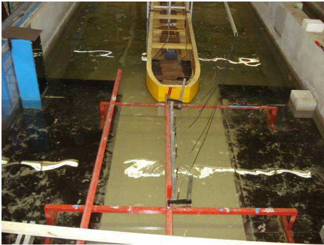
Figure 1: View of the basin, vessel, and sediment bed.
