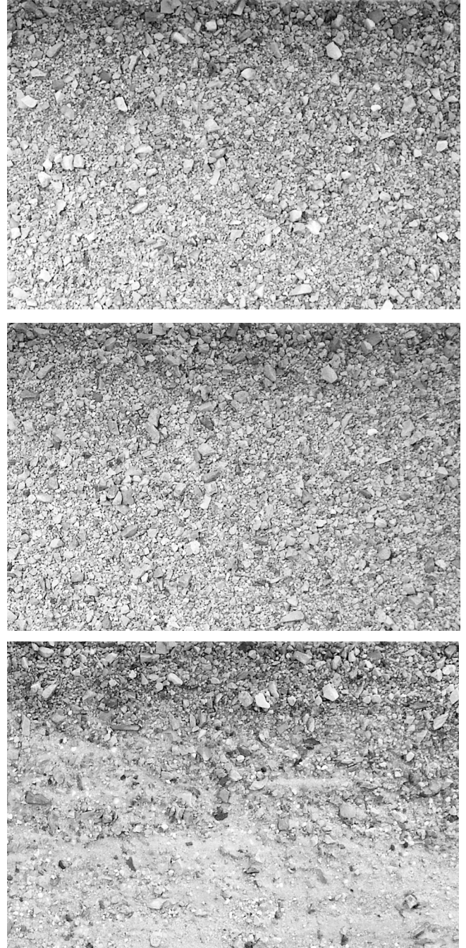
Figure 7: Rip rap in the flume (same 20 m long area as in figure 4) after shear stresses of 156 N/m 2 (top), 178 N/m 2 (middle) and 193 N/m 2 (bottom), flow direction from left to right
