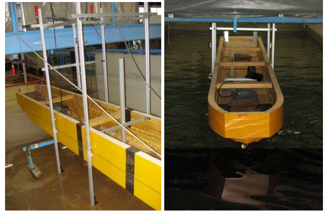
Figure 2: Detailed view of the ship's holding frame (left: in dry conditions; right: during vessel operation).
