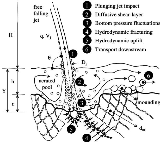
Figure 1: Main parameters and physical-mechanical processes (Bollaert, 2002)
