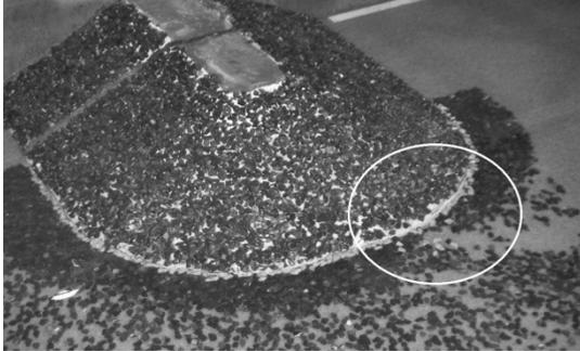
Figure 2 Apron configuration after a failure test (yellow painted stones dislodged in the encircled zone)
