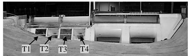
Figure 1: A photograph with the HPP model structure; there are 4 intakes on the left bottom, 2 outlets on the right bottom and 4 flap gates on the top part of the plant.
