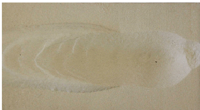
Figure 10: Scour geometry resulting from Wageningen-propeller with central rudder.
