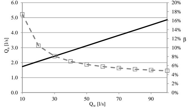
Figure 4: Passively entrained air discharge (black line) and air-water ratio (dashed grey line) as a function of the water jet discharge
