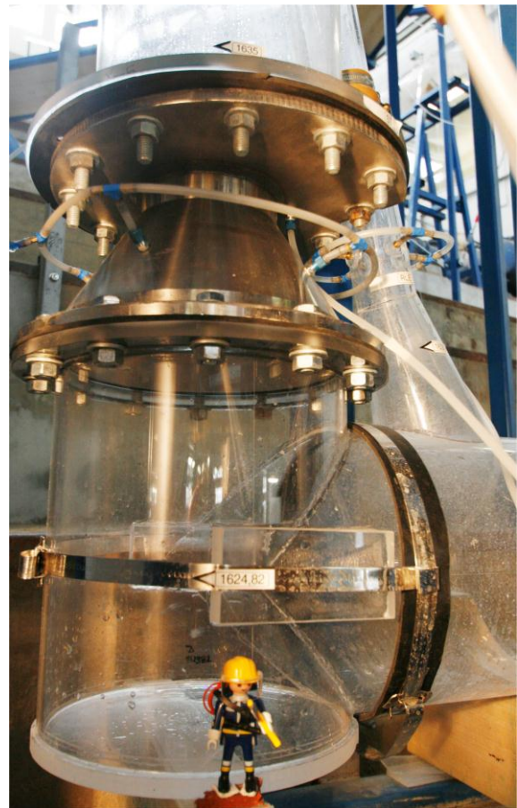
Figure 8: Asymmetric Throttle at end of lower chamber with scaled model figure
