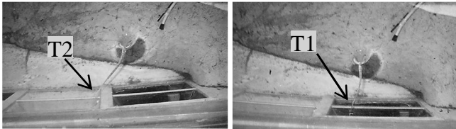
Figure 5: Intake vortex at turbine combination ‘B0’; the air core entered the T1 and T2 alternately.
