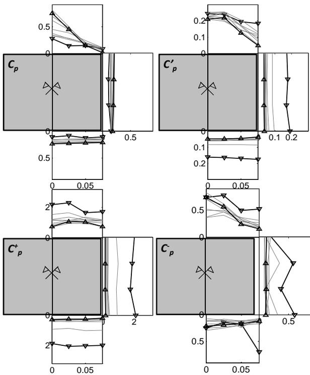
Figure 6: Scaled plots of  $C_p$ ,  $C_p'$ ,  $C_p^+$  and  $C_p^-$  for all  $V_j$  around block. Downward triangle:  $V_j = 2.46$  m/s. Upward triangle:  $V_j = 21.14$  m/s. Intermediate values in grey. Aerated test,  $Y/D_j = 6.94$ .
