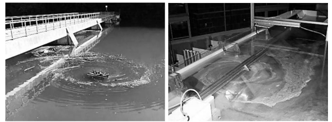
Figure 3: Photographs showing a good match of the intake free surface vortex on the HPP Fluhmühle (left) and of its model (right) with the land side turbine in operation only.
