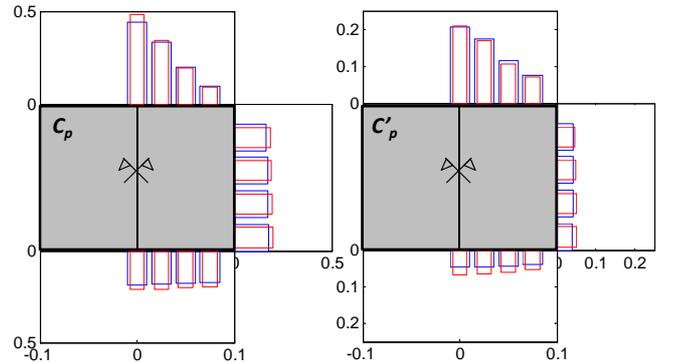
Figure 5: Scaled plots of  $C_p$  and  $C_p'$  around block.  $Y/D_j=11.11$ ;  $V_j=19.65$ m/s. Red: without air. Blue: with air.
