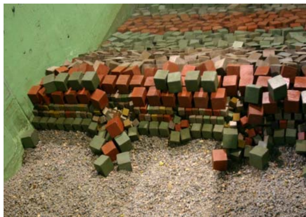
Figure 14. Stage 2. Final situation ( H_s = 11 m, T_p = 20 s).
