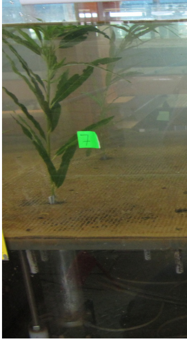
Figure 2. A Salix viminalis specimen attached to the drag force sensor located below the flume bottom.
