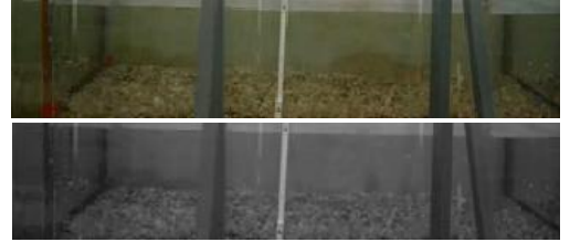
Figure 8: Frame #10 from test video (above) and estimated background using pixel-wise median filtering (below).
