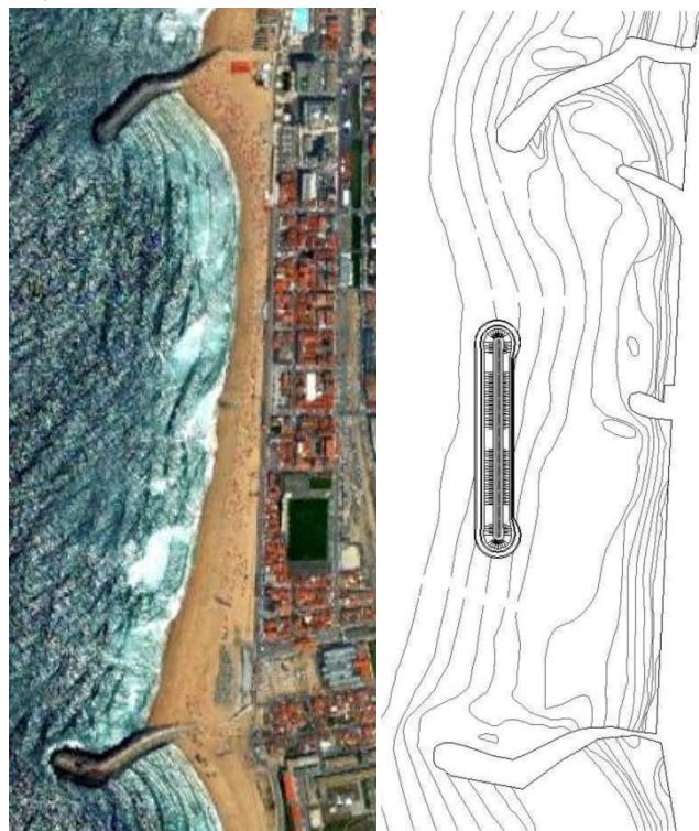
Figure 1: Espinho urban front in July 2010 (left, Google Earth TM ). Detached breakwater proposed by Pereira (2008) (right, schematic representation).
