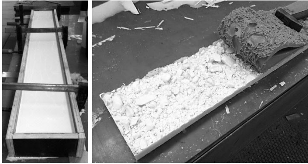
Figure 2: left : filled casting form ; right : detaching
