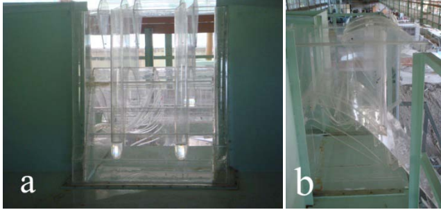
Figure 2: Spillway crest of the physical model: a) View from the reservoir, b) Side view.
